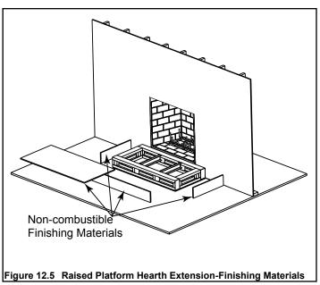
Hearths should slope away from the front of the fireplace and chase at 1/8 in. to 1/4 in. per foot. Spark strips must be on top of any combustible hearth materials used for moisture management.
